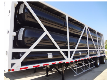
Figure 4: Hydrogen trailer with large storage tanks. Source: Hexagon
